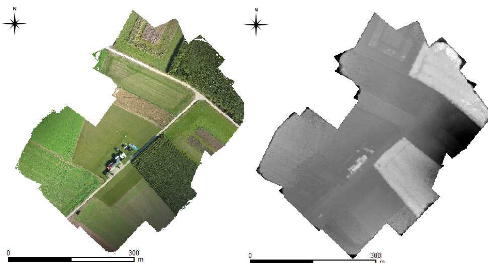
Figure 1. Orthomosaic (left) and Digital Elevation Model (right) based on imagery acquired from the USENSE-X8 UAV
